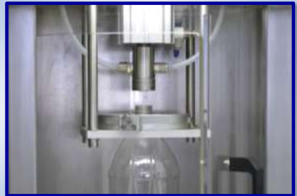
Automatic filling system
