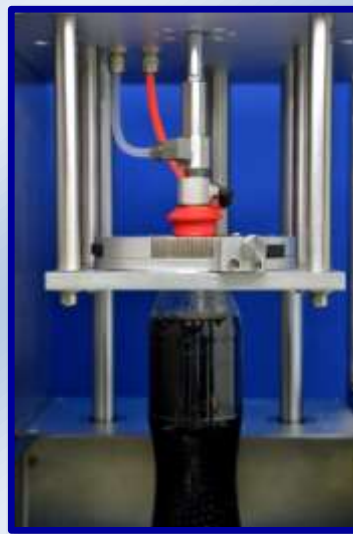
Automated piercing and testing with AT2E patent needle
