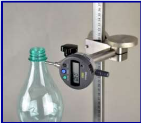
Ruler allows accurate measuring position
