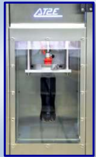
Automated piercing and testing with AT2E patent needle
