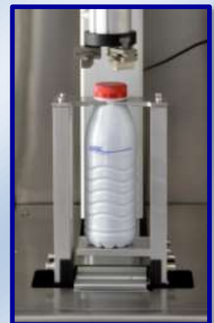
Automatic squeezing clamping system for PET packaging (Optional)
