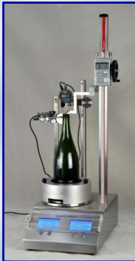
UBPT-3 with 3 measuring heads (for mouth clearance, perpendicularity & height) and integrated double automatic calculators
