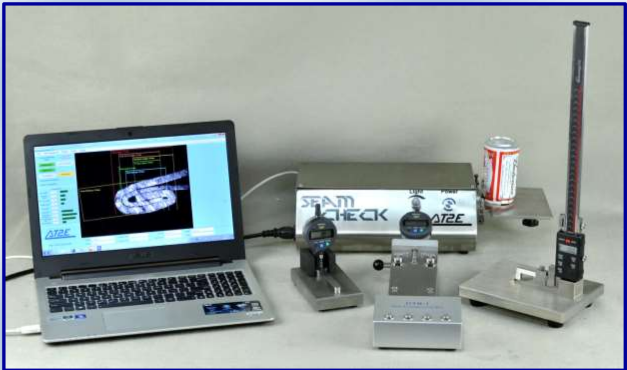
SeamCheck connecting with optional gauges through DTB-1
